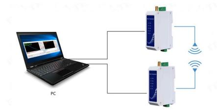
④ Start two serial port debugging assistants, select the serial port baud rate to be 9600bps (default), and the check method to be 8N1 to realize serial port transparent transmission;
