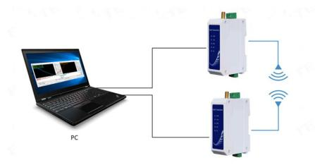
④ Start two serial port debugging assistants, select the serial port baud rate to be 9600bps (default), and the check
