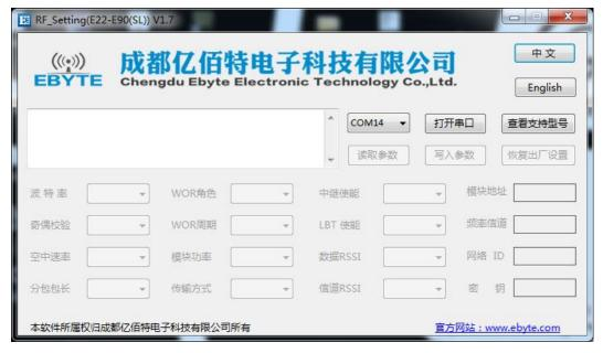
In the configuration of the host computer, the module address, frequency channel, network ID, and key are in decimal display mode, where each parameter takes a range of values:
