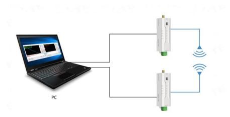
General port debugging assistant, select serial port port rate of 9600bps (default), check mode of 8N1, can achieve serial port transmission;
