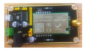
As shown in the figure, plug in the jumper cap ( choose 3.3 V power supply, mode 0), the two Test kits are configured in this way, open the corresponding serial port, you can send and receive data, and you can observe the flickering of the AUX light on the bottom board.
