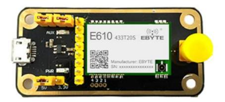
As shown in the figure, plug in the jumper cap ( choose 3.3 V power supply, mode 0), the two EXX-XXXTBH-01 are configured in this way, open the corresponding serial port, you can send and receive data, and you can observe the flickering of the AUX light on the bottom board.
