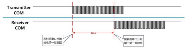
Data delay schematic (at a serial port baud rate of 115200, sending 22 bytes)
