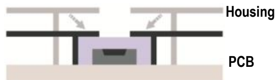
Figure 13. Small measurement dead zone helps the sensor to quickly and comprehensively detect environmental changes.
